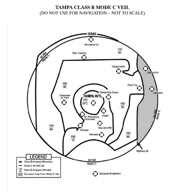
Operators of aircraft not equipped with Mode C transponders may operate within the Tampa Class B Mode C veil to attend the Sun 'n Fun Fly–In at LAL along the following ATC-designated route:
